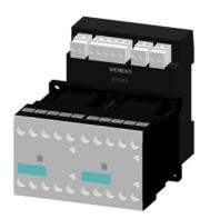
SIRIUS safety relay with contactor relay enabling circuits (EC) 230 V DC, 90 mm Screw terminal EC instantaneous: 3 NO EC delayed: 0 SC: 0 Autostart/monitored start Basic device Maximum achieved SIL: 2, PL: d
