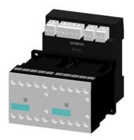
SIRIUS safety relay with contactor relay enabling circuits (EC) 24 V DC, 90 mm Screw terminal EC instantaneous: 2 NO EC delayed: 0 SC: 1NC Autostart/monitored start Basic device Maximum achieved SIL: 2, PL: d
