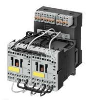
SIRIUS safety relay with contactor relay enabling circuits (EC) 24 V DC, 90 mm Spring-type terminal EC instantaneous: 2 NO EC delayed: 0 SC: 1NC Autostart/monitored start Basic device Maximum achieved SIL: 2, PL: d
