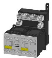
SIRIUS safety relay with contactor relay enabling circuits (EC) 24 V DC, 90 mm Screw terminal EC instantaneous: 3 NO + 1 HL EC delayed: 0 SC: 0 Autostart/monitored start Basic device Maximum achieved SIL: 3, PL: e
