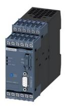
Basic unit SIMOCODE pro V PB PROFIBUS DP interface 12 Mbit/s, RS 485, 41/30 freely parameterizable, Us: 24 V DC, input for thermistor connection Monostable relay outputs, expandable by extension modules
