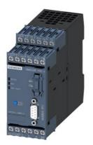
Basic unit SIMOCODE pro V MR, MODBUS RTU interface 57.6 Kbps, RS 485, 4I/3O freely parameterizable, Us: 24 V DC, input for thermistor connection Monostable relay outputs, expandable by extension modules
