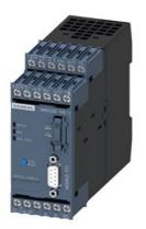
Basic unit SIMOCODE pro V MR, MODBUS RTU interface 57.6 Kbps, RS 485, 4l/3O freely parameterizable, Us: 110...240 V AC/DC, input for thermistor connection Monostable relay outputs, expandable by extension modules
