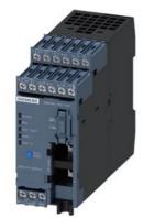
Basic unit SIMOCODE pro V EIP, EtherNet/IP, medium redundancy DLR, Web server, transmission rate 100 Mbps, 2 x bus connection via RJ45, 4I/30 freely parameterizable, Us: 110...240 V AC/DC, input for thermistor connection Monostable relay outputs, expandable by extension modules
