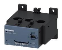
Current/voltage measuring module Set current 20...200 A voltage measurement up to 690 V, overall width 120 mm, straight-through transformer
