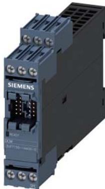
Decoupling module for installation upstream of the current/voltage measuring module at the system interface for application in ungrounded supply systems
