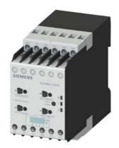
Insulation monitoring relay for ungrounded (IT) supply systems up to 400 V AC, 15-400 Hz and up to 600 V DC Measuring range 1-100 / 2-200 kohm Supply voltage 24-240 V AC/DC Width 45 mm 1 + 1 or 2 change-over contacts screw terminal
