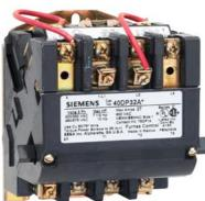
Non-reversing NEMA contactor, Size 0, Three phase full voltage, Contactor amp rating 18A, 3 wire (NO aux included), 110-120/220-240VAC 60Hz coil, Non-combination type, Enclosure NEMA type (open), No enclosure
