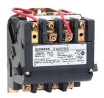
Non-reversing NEMA contactor, Size 1, Three phase full voltage, Contactor amp rating 27A, 3 wire (NO aux included), 208VAC 60Hz coil, Non-combination type, Enclosure NEMA type (open), No enclosure
