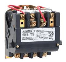
Non-reversing NEMA contactor, Size 1, Three phase full voltage, Contactor amp rating 27A, 3 wire (NO aux included), 110V 50Hz / 120V 60Hz coil, Non-combination type, Enclosure NEMA type (open), No enclosure
