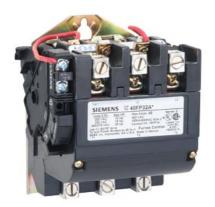
Non-reversing NEMA contactor, Size 2, Three phase full voltage, Contactor amprating 45A, 3 wire (NO aux included), 110-120/220-240VAC 60Hz coil, Noncombination type, Enclosure NEMA type (open), No enclosure
