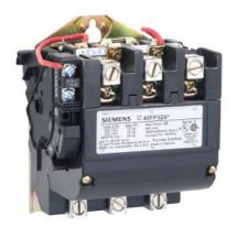
Non-reversing NEMA contactor, Size 2, Three phase full voltage, Contactor amp rating 45A, 3 wire (NO aux included), 208VAC 60Hz coil, Non-combination type, Enclosure NEMA type (open), No enclosure
