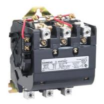
Non-reversing NEMA contactor, Size 3, Three phase full voltage, Contactor amprating 90A, 3 wire (NO aux included), 110V 50Hz / 120V 60Hz coil, Noncombination type, Enclosure NEMA type (open), No enclosure
