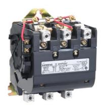
Non-reversing contactor, Size 3 1/2, Three phase full voltage, Contactor amp rating 115A, 3 wire (NO aux included), 110-120/220-240VAC 60Hz coil, Non-combination type, Enclosure NEMA type (open), No enclosure
