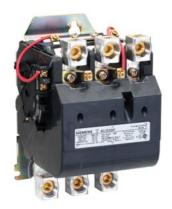
Non-reversing NEMA contactor, Size 4, Three phase full voltage, Contactor amp rating 135A, 3 wire (NO aux included), 110-120/220-240VAC 60Hz coil, Non-combination type, Enclosure NEMA type (open), No enclosure
