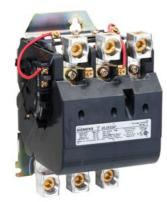
Non-reversing NEMA contactor, Size 4, Three phase full voltage, Contactor amp rating 135A, 3 wire (NO aux included), 110V 50Hz / 120V 60Hz coil, Noncombination type, Enclosure NEMA type (open), No enclosure
