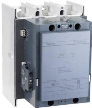
Non-reversing NEMA contactor, Size 7, Three phase full voltage, Contactor amp rating 810A, 3 wire (NO aux included), 150-500V 50-60Hz/DC coil, Non-combination type, Enclosure NEMA type (open), No enclosure
