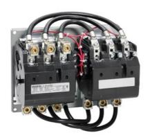
Reversing NEMA contactor Size 4 Three phase full voltage Contactor amp rating 135Amp 3 110V 50HZ / 120V 60HZ coil Non-combination type Enclosure NEMA type (open) No enclosure
