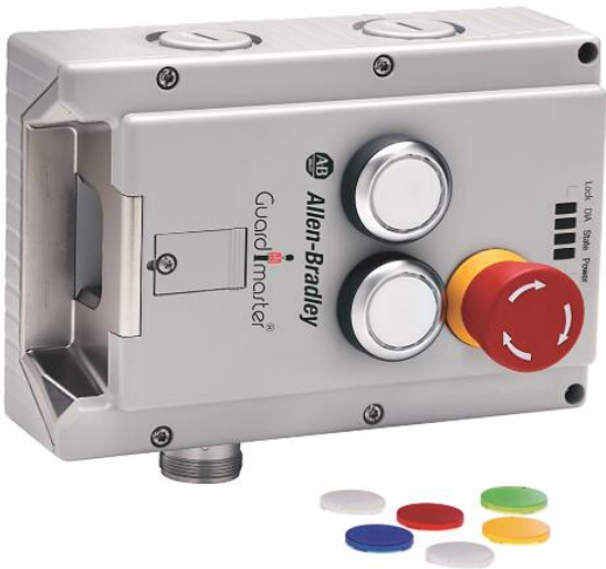
442G Access Box Lock Module, Power to Release, M23 Left Guard, Emergency Stop & 2 Pushbuttons
