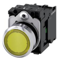
Illuminated pushbutton, 22 mm, round, metal, shiny, yellow, pushbutton, flat, momentary contact type, with holder, 1NO, LED module with integrated LED 110 V AC, screw terminal, with laser labeling, symbol number according to, ISO 7000 or IEC 60417
