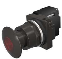
30mm BlackMax, Epoxy Coated Corrosion Resistant Complete Metal Unit Illuminated Push-Pull Operator Full Voltage, 120V AC/DC LED Lamp Mushroom Head Cap Small 1 3/4" (44.5 mm) Metal, Black with Red Lens 3 Position Momentary UL Listed, CSA Certified NEMA 1,3,3R,4,4X,12,13 & Automotive Standards
