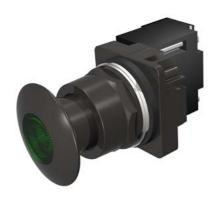
30mm BlackMax, Epoxy Coated Corrosion Resistant Complete Metal Unit Illuminated Push-Pull Operator Full Voltage, 120V AC/DC LED Lamp Mushroom Head Cap Small 1 3/4" (44.5 mm) Metal, Black with Green Lens 3 Position Momentary UL Listed, CSA Certified NEMA 1,3,3R,4,4X,12,13 & Automotive Standards
