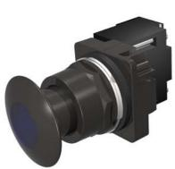
30mm BlackMax, Epoxy Coated Corrosion Resistant Complete Metal Unit Illuminated Push-Pull Operator Full Voltage, 120V AC/DC Incandescent Lamp Mushroom Head Cap Small 1 3/4" (44.5 mm) Metal, Black with Blue Lens 3 Position Momentary UL Listed, CSA Certified NEMA 1,3,3R,4,4X,12,13 & Automotive Standards
