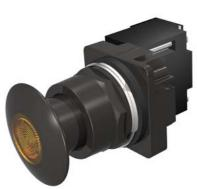
30mm BlackMax, Epoxy Coated Corrosion Resistant Complete Metal Unit Illuminated Push-Pull Operator Transformer type, 120V AC Incandescent Lamp Mushroom Head Cap Small 1 3/4" (44.5 mm) Metal, Black with Amber Lens 3 Position Momentary UL Listed, CSA Certified NEMA 1,3,3R,4,4X,12,13 & Automotive Standards
