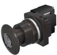
30mm BlackMax, Epoxy Coated Corrosion Resistant Complete Metal Unit Illuminated Push-Pull Operator Transformer type, 120V AC Incandescent Lamp Mushroom Head Cap Small 1 3/4" (44.5 mm) Metal, Black with Clear Lens 3 Position Momentary UL Listed, CSA Certified NEMA 1,3,3R,4,4X,12,13 & Automotive Standards
