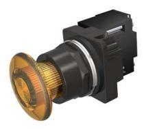
30mm BlackMax, Epoxy Coated Corrosion Resistant Complete Metal Unit Illuminated Push-Pull Operator Transformer type, 120V AC Incandescent Lamp Mushroom Head Cap Small 1 3/4" (44.5 mm) Plastic, Amber 3 Position Momentary UL Listed, CSA Certified NEMA 1,3,3R,4,4X,12,13 & Automotive Standards
