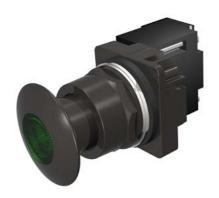
30mm BlackMax, Epoxy Coated Corrosion Resistant Complete Metal Unit Illuminated Push-Pull Operator Transformer type, 240V AC Incandescent Lamp Mushroom Head Cap Small 1 3/4" (44.5 mm) Metal, Black with Green Lens 3 Position Momentary UL Listed, CSA Certified NEMA 1,3,3R,4,4X,12,13 & Automotive Standards
