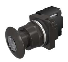
30mm BlackMax, Epoxy Coated Corrosion Resistant Complete Metal Unit Illuminated Push-Pull Operator Transformer type, 600V AC LED Lamp Mushroom Head Cap Small 1 3/4" (44.5 mm) Metal, Black with Clear Lens 3 Position Momentary UL Listed, CSA Certified NEMA 1,3,3R,4,4X,12,13 & Automotive Standards
