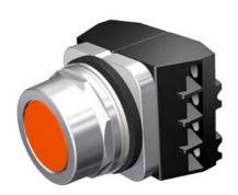
30mm Command/52, Chrome Finish Heavy Duty, Watertight/Oiltight Complete Metal Unit Pushbutton Non-Illuminated Flush Button Plastic Cap, Orange 2 Position Momentary with 2 N.O. - 2 N.C. Heavy Duty Contacts, A600/P600 UL Listed, CSA Certified NEMA 1,3,3R,4,4X,12,13 & Automotive Standards
