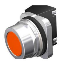
30mm Command/52, Chrome Finish Heavy Duty, Watertight/Oiltight Complete Metal Unit Pushbutton Non-Illuminated Flush Button Plastic Cap, Orange 2 Position Momentary with 1 N.C. Late Break Heavy Duty Contacts, A600/P600 UL Listed, CSA Certified NEMA 1,3,3R,4,4X,12,13 & Automotive Standards
