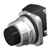
30mm Command/52, Chrome Finish Heavy Duty, Watertight/Oiltight Complete Metal Unit Pushbutton Non-Illuminated Extended Button Plastic Cap, Black 2 Position Momentary with 1 N.C. Late Break Heavy Duty Contacts, A600/P600 UL Listed, CSA Certified NEMA 1,3,3R,4,4X,12,13 & Automotive Standards
