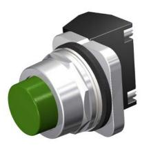
Metal, pushbutton 2 position, 1NO-1NC Complete device Momentary Extended, green Non-Illuminated UL file E22655 in Vol. 6 (7) Sec. 13 (2)
