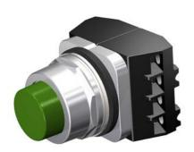
30mm Command/52, Chrome Finish Heavy Duty, Watertight/Oiltight Complete Metal Unit Pushbutton Non-Illuminated Extended Button Plastic Cap, Green 2 Position Momentary with 2 N.C. Heavy Duty Contacts, A600/P600 UL Listed, CSA Certified NEMA 1,3,3R,4,4X,12,13 & Automotive Standards
