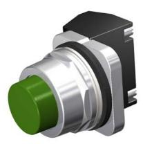
30mm Command/52, Chrome Finish Heavy Duty,Watertight/Oiltight Complete Metal Unit Pushbutton Non-Illuminated Extended Button Plastic Cap, Green 2 Position Momentary with 1 N.O. Early Make Heavy Duty Contacts, A600/P600 UL Listed, CSA Certified NEMA 1,3,3R,4,4X,12,13 & Automotive Standards
