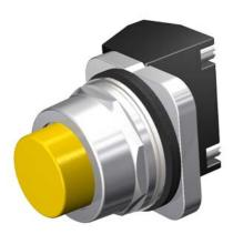
30mm Command/52, Chrome Finish Heavy Duty, Watertight/Oiltight Complete Metal Unit Pushbutton Non-Illuminated Extended Button Plastic Cap, Yellow 2 Position Momentary with 1 N.O. - 1 N.C. Heavy Duty Contacts, A600/P600 UL Listed, CSA Certified NEMA 1,3,3R,4,4X,12,13 & Automotive Standards
