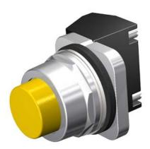
30mm Command/52, Chrome Finish Heavy Duty, Watertight/Oiltight Complete Metal Unit Pushbutton Non-Illuminated Extended Button Plastic Cap, Yellow 2 Position Momentary with 1 N.C. Late Break Heavy Duty Contacts, A600/P600 UL Listed, CSA Certified NEMA 1,3,3R,4,4X,12,13 & Automotive Standards
