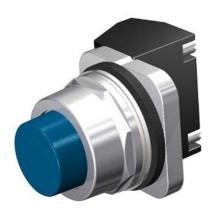
30mm Command/52, Chrome Finish Heavy Duty, Watertight/Oiltight Complete Metal Unit Pushbutton Non-Illuminated Extended Button Plastic Cap, Blue 2 Position Momentary with 1 N.C. Late Break Heavy Duty Contacts, A600/P600 UL Listed, CSA Certified NEMA 1,3,3R,4,4X,12,13 & Automotive Standards
