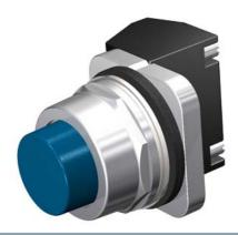
30mm Command/52, Chrome Finish Heavy Duty, Watertight/Oiltight Complete Metal Unit Pushbutton Non-Illuminated Extended Button Plastic Cap, Blue 2 Position Momentary with 1 N.O. Early Make Heavy Duty Contacts, A600/P600 UL Listed, CSA Certified NEMA 1,3,3R,4,4X,12,13 & Automotive Standards
