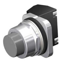
30mm Command/52, Chrome Finish Heavy Duty,Watertight/Oiltight Complete Metal Unit Pushbutton Non-Illuminated Extended Button Plastic Cap, Gray 2 Position Momentary with 1 N.O. - 1 N.C. Heavy Duty Contacts, A600/P600 UL Listed, CSA Certified NEMA 1,3,3R,4,4X,12,13 & Automotive Standards
