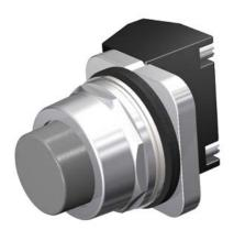
30mm Command/52, Chrome Finish Heavy Duty, Watertight/Oiltight Complete Metal Unit Pushbutton Non-Illuminated Extended Button Plastic Cap, Gray 2 Position Momentary with 1 N.O. Early Make Heavy Duty Contacts, A600/P600 UL Listed, CSA Certified NEMA 1,3,3R,4,4X,12,13 & Automotive Standards
