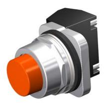
30mm Command/52, Chrome Finish Heavy Duty,Watertight/Oiltight Complete Metal Unit Pushbutton Non-Illuminated Extended Button Plastic Cap, Orange 2 Position Momentary with 1 N.C. Late Break Heavy Duty Contacts, A600/P600 UL Listed, CSA Certified NEMA 1,3,3R,4,4X,12,13 & Automotive Standards
