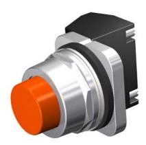
30mm Command/52, Chrome Finish Heavy Duty, Watertight/Oiltight Complete Metal Unit Pushbutton Non-Illuminated Extended Button Plastic Cap, Orange 2 Position Momentary with 1 N.C. Heavy Duty Contacts, A600/P600 UL Listed, CSA Certified NEMA 1,3,3R,4,4X,12,13 & Automotive Standards
