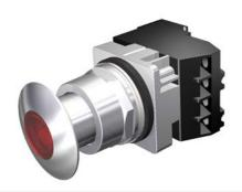
30mm Command/52, Chrome Finish Heavy Duty, Watertight/Oiltight Complete Metal Unit Illuminated Push-Pull Operator Full Voltage, 6V AC LED Lamp Mushroom Head Cap Small 1 3/4" (44.5 mm) Metal, Chrome with Red Lens 2 Position Maintained, Pull-to-Release with 1 N.O. - 1 N.C. Heavy Duty Contacts, A600/P600 UL Listed, CSA Certified NEMA 1,3,3R,4,4X,12,13 & Automotive Standards
