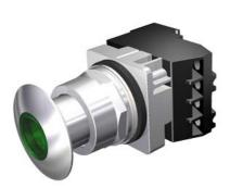
30mm Command/52, Chrome Finish Heavy Duty,Watertight/Oiltight Complete Metal Unit Illuminated Push-Pull Operator Full Voltage, 6V AC LED Lamp Mushroom Head Cap Small 1 3/4" (44.5 mm) Metal, Chrome with Green Lens 2 Position Maintained, Pull-to-Release with 1 N.O. - 1 N.C. Heavy Duty Contacts, A600/P600 UL Listed, CSA Certified NEMA 1,3,3R,4,4X,12,13 & Automotive Standards
