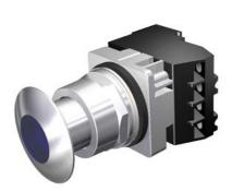
30mm Command/52, Chrome Finish Heavy Duty,Watertight/Oiltight Complete Metal Unit Illuminated Push-Pull Operator Full Voltage, 6V AC LED Lamp Mushroom Head Cap Small 1 3/4" (44.5 mm) Metal, Chrome with Blue Lens 2 Position Maintained, Pull-to-Release with 1 N.O. - 1 N.C. Heavy Duty Contacts, A600/P600 UL Listed, CSA Certified NEMA 1,3,3R,4,4X,12,13 & Automotive Standards
