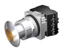
30mm Command/52, Chrome Finish Heavy Duty, Watertight/Oiltight Complete Metal Unit Illuminated Push-Pull Operator Full Voltage, 6V AC LED Lamp Mushroom Head Cap Small 1 3/4" (44.5 mm) Metal, Chrome with Amber Lens 2 Position Maintained, Pull-to-Release with 1 N.O. - 1 N.C. Heavy Duty Contacts, A600/P600 UL Listed, CSA Certified NEMA 1,3,3R,4,4X,12,13 & Automotive Standards
